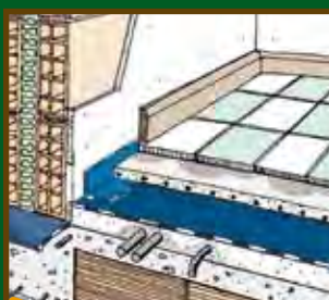
Acoustic insulation of floor against foot-traffic noise
