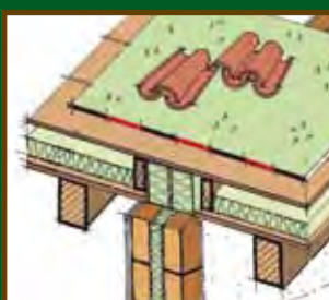
Thermal and acoustic insulation of roofs against airborne noise
