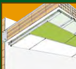
Thermal and acoustic insulation of ceilings against airborne and foot-traffic noise
